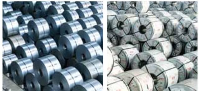
**8** As for formed steel, the slabs are transferred to the hot rolling mills while the billets are transferred to the wired rod mill. The coils and sheets are flat steel products made from slabs, whereas, wired rods, a kind of long product, is derived from billets.
